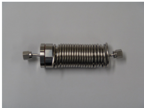
Fig. 4. Photograph of PROX reactor with coiled heat-exchanger (34 cm 3 , 25 mm outer diameter \times 70 mm length.).
